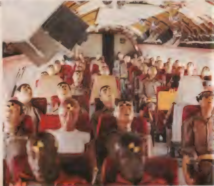
One-way trip: dozens of dummy passengers, some fitted with electronic impact sensors, await takeoff
